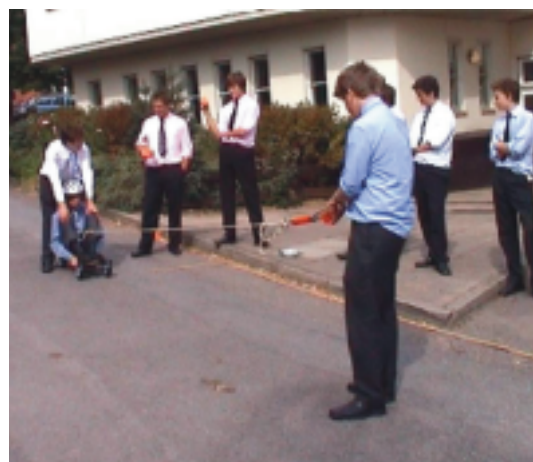
Figure 2 The basic set up for testing F = ma (NB. rope should pull parallel with road, not sloping up, as shown here).
